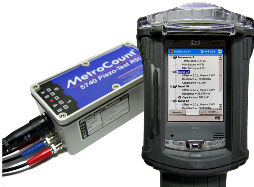
Checking piezo sensors with an MC5740 and Pocket PC
